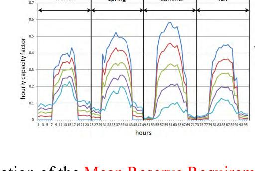
Variation of the Mean Reserve Requirements for Sites A, B and C for 20% penetration level.  $P_H > P_{LD} \sim \text{power export}; P_H < P_{LD} \sim \text{power import}$ Case II/ III give minimum reserve requirements for the different sites; leads to suitable sizing.
