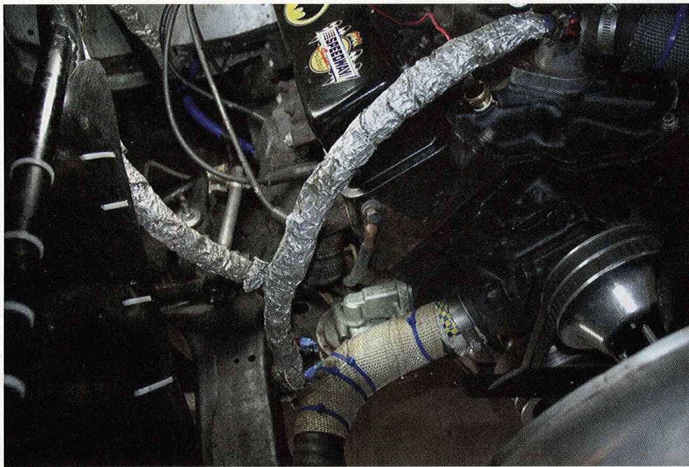
An experiment with under-hood heat management led Lograsso to insulate his lower radiator hose, and insulate and foil-wrap his fuel lines to keep fuel cooler on its way to the carburetor.
